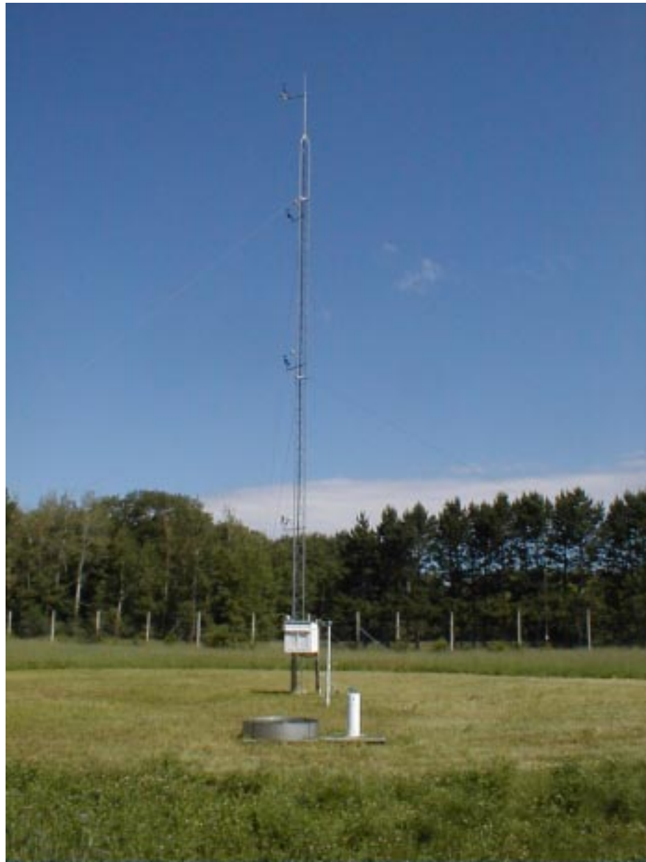
Figure 10.—Aspen FACE meteorological tower containing instruments to measure site background meteorological parameters (see table 3).
