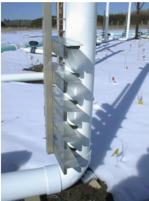
Figure 13.—Individual treatment ring gas distribution equipment. A. Control shed, gas injection fan, and connecting plenum pipe. B. Butterfly control valves. C. Vertical vent pipe with gas emitter ports and baffles.
