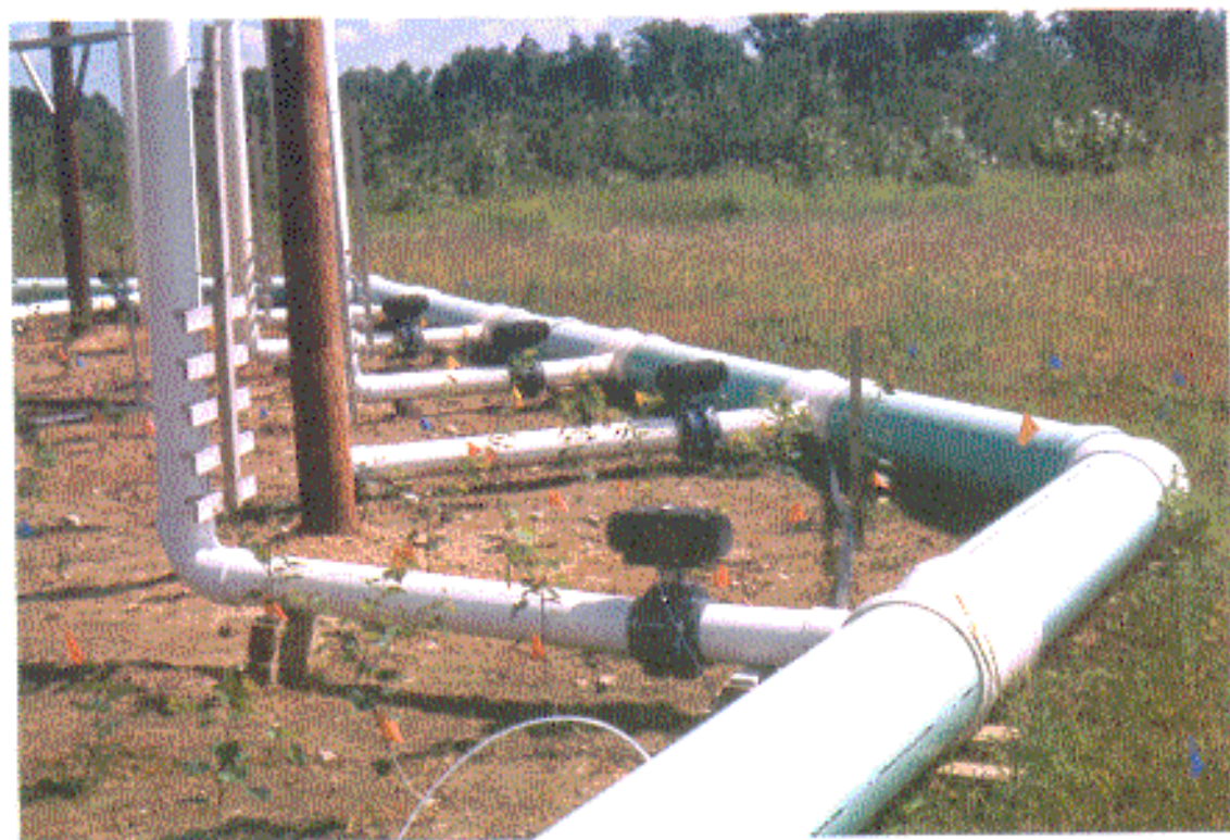
Figure 12.—Individual treatment ring configuration in 1997 showing: A. Octagon plenum pipe, vertical vent pipes, support poles, crosswalks, and control shed. B. Octagon plenum pipe, vertical vent pipes, and butterfly control valves. C. Treatment ring in 1999 with increased tree growth and extensions on the vertical vent pipes.
